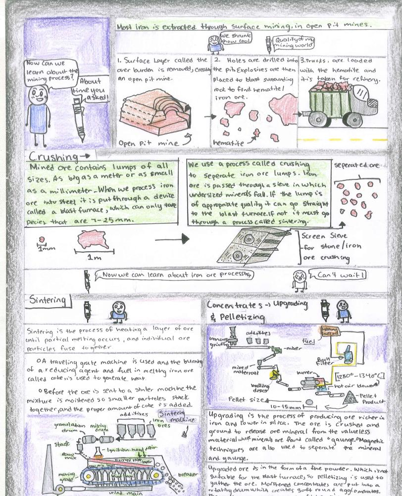
The balls are hardened by firing air.
